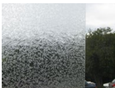
Glue-Chip Available in 3mm and 5mm thickness and is also laminated 5mm can be toughened
